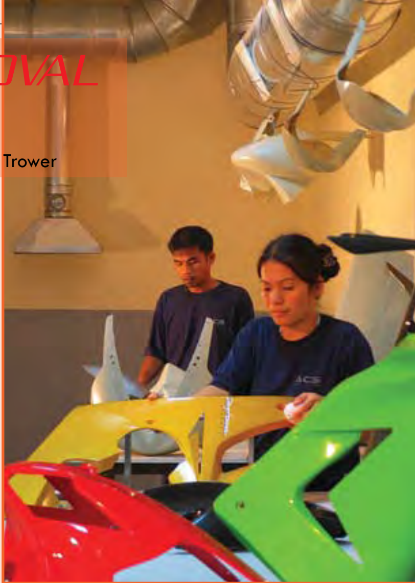
Joy Aspe (background) supervises the hand finishing of kevlar motorbike fairings produced at a ACS's new factory, located in the SRF Compound, Subic Bay Freeport Zone. Photo by Kevin Hamdorf.
